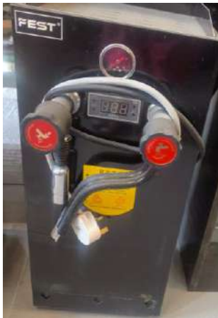
17. FEST-RC-800-H HIGH PRESSURE MILK STEAMER
